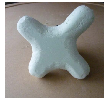
Design of the controller. This was inspired by the traditional wooden control of a marionette. The idea was that it could be tilted to move Ami.
