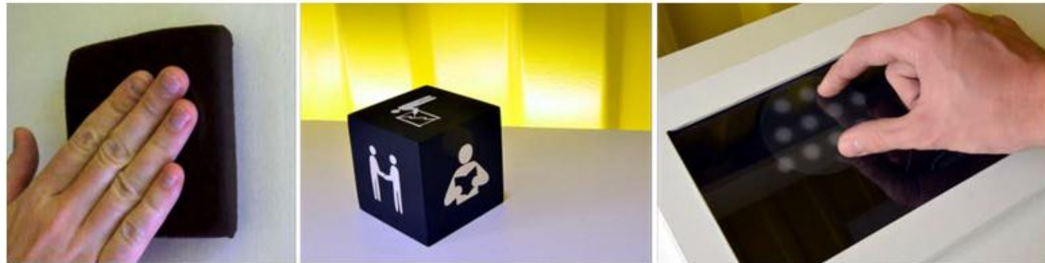
figure 2. Three existing Interfaces for Breakout404; with varying levels of control; expressive atmosphere setting with the LightPad , calling presets with the LightCube , and detailed control with a tablet interface.
